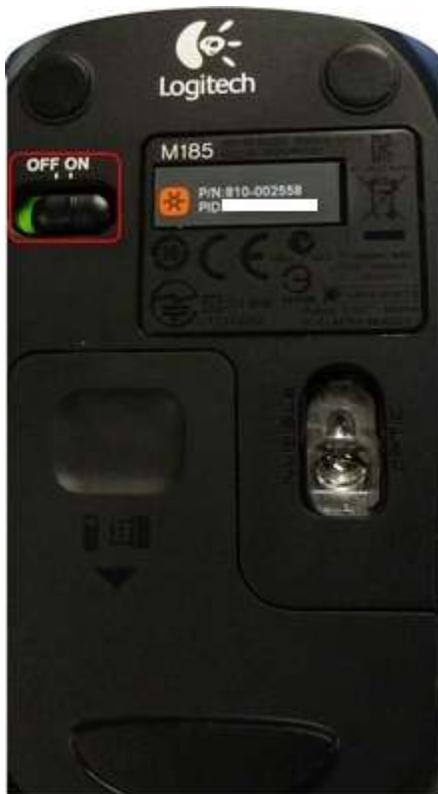
Your mouse uses an infrared (IR) optical LED light that is invisible to the human eye. This means you won't be able to see the light emitting from the bottom of your mouse.
