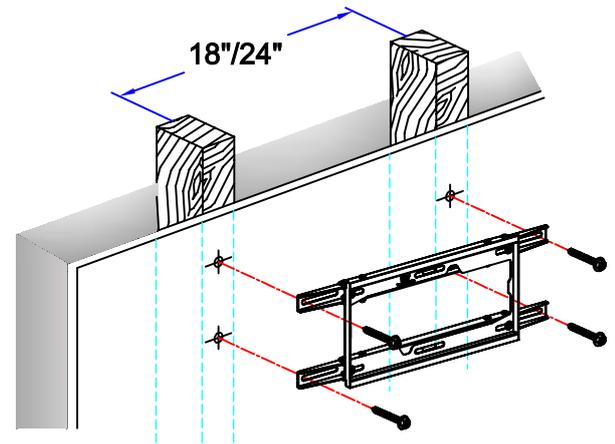
Solution 3. If studs spacing is over 16" (less than 24") or not in your desired position, apply 24" extension plate MD5232 (available on Amazon.com) to bridge up wood studs up to 24".
